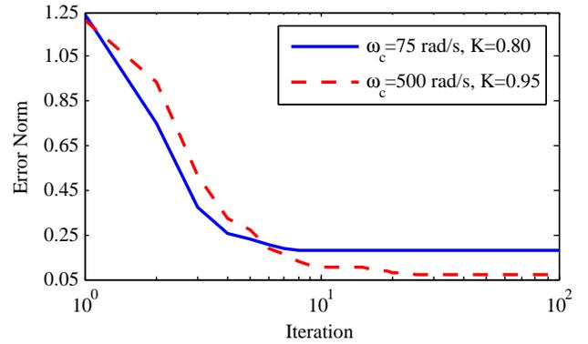
Fig. 3: Effect of  $Q$  and  $\mathcal{L}_1$  filter bandwidths on learning performance
