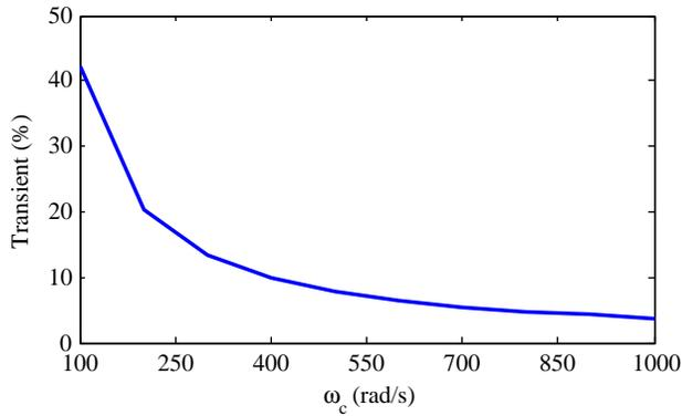
Fig. 6: Effect of the feedback filter bandwidth on system transients with  $K = 0.80$
