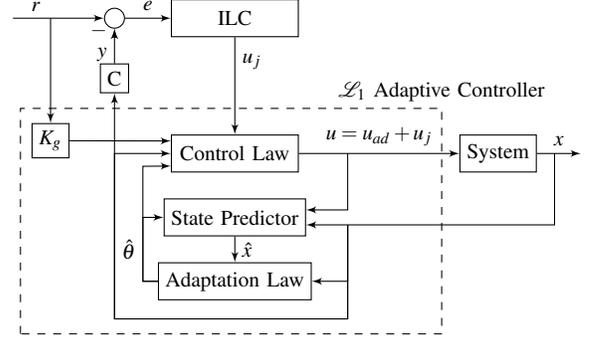
Fig. 1: ILC with modified  $\mathcal{L}_1$  adaptive feedback
