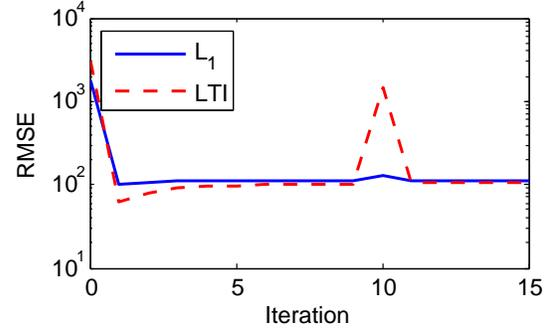
FIGURE 2. Transients in the learning controllers due to change of parameters. Scenario 1.
