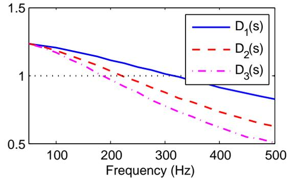
FIGURE 1.  $L_1$  stability condition as a function of cutoff frequency for different filters. Here,  $D_1(s) = 1 - \left(\frac{s}{s+2\pi f_c}\right)$ ,  $D_2(s) = 1 - \left(\frac{s}{s+2\pi f_c}\right)^2$ , and  $D_3(s) = 1 - \left(\frac{s}{s+2\pi f_c}\right)^3$ .
